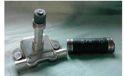
*Wheelbox removed from the car shown with heater hose*
