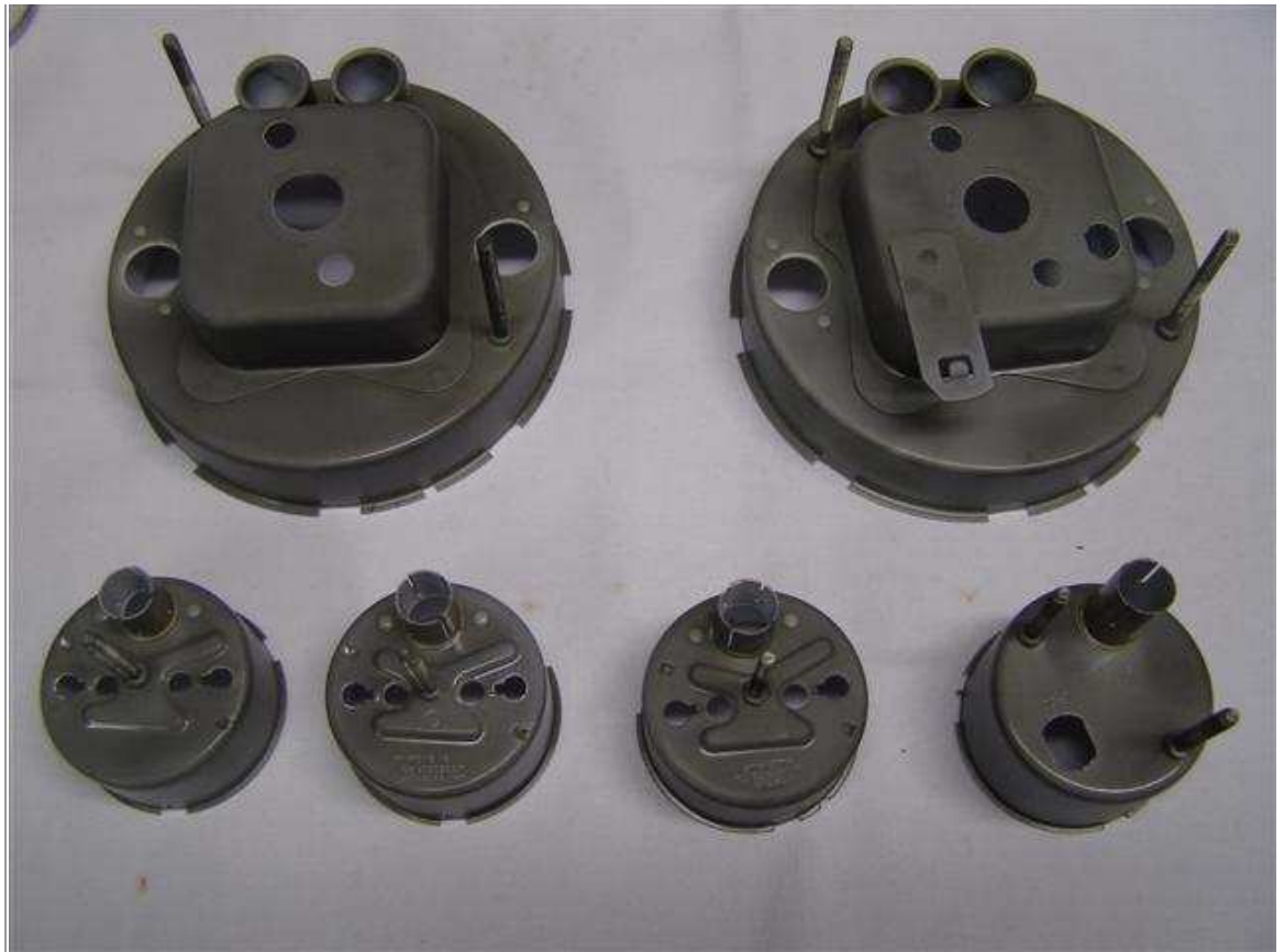
Two coats of Rustoleum One Step Clear sealed these up nicely.
