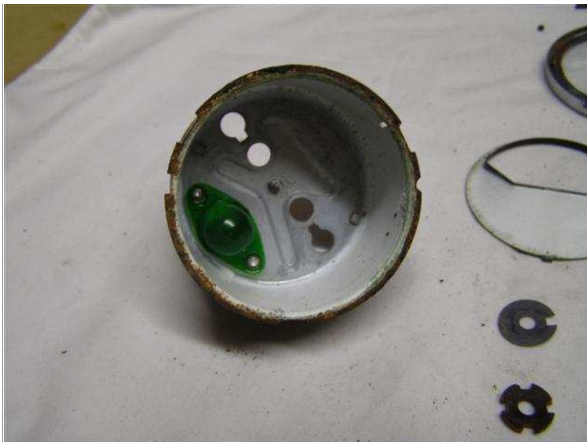
The case is now empty and ready for bead blasting.
