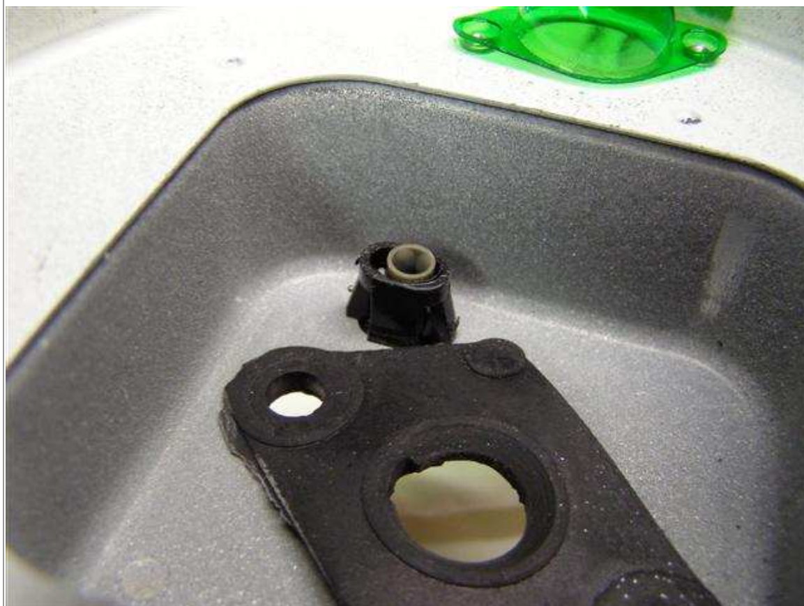
This is how the Odometer Reset Cable is removed. Yes, it's a pain, but Smith did this not Lucas.
