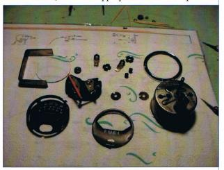
of the disassembly taking care once again with the movement and inner face. You'll probably need to replace the O-rings. I purchased new ones from Barrie Robinson in Canada. He sells a complete set for the Tiger that consists of 14 O-rings (2 large & 4 small Jaeger's gauges) for US\$17 including postage.
