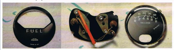
To remove the inner face, you'll need to take it out at the same time as the movement itself. The needle is very fragile, so care must be taken to keep it from bending. Unscrew the 2 slotted barrel nuts on the back of the gauge and work the inner face out of the housing while holding it face down. This will allow the movement to fall free and be supported by the face with no load on the needle assembly. Once removed, gently slide the needle and movement out from the face.
